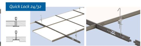
24 mm wide base system for lay-in and rebated edge panels
