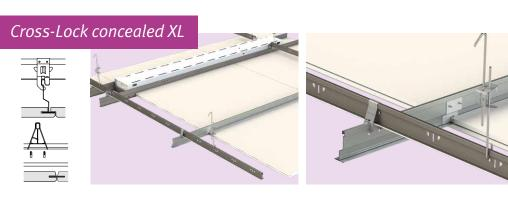
system for concealed installation of large size panels
