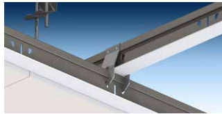
Cross-Lock concealed suspension system - Stable, dimensionally accurate, XL for large-format panels.
